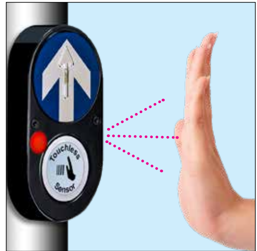
Sensor Activation between 5 – 15cm
