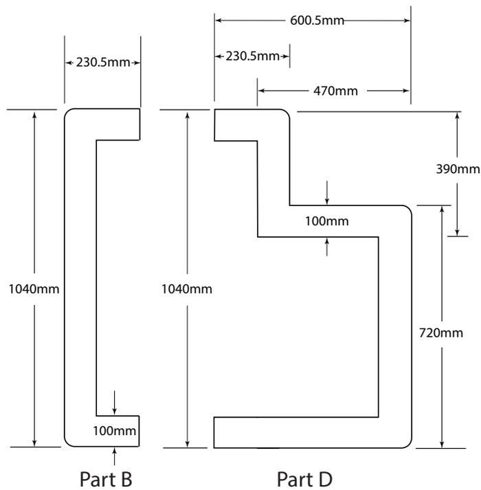
Backing board made up of 2 x sections (Part B) 230.5 x x1040mm + (Part D) 600.5 mm x 1040 mm and 4mm thick
