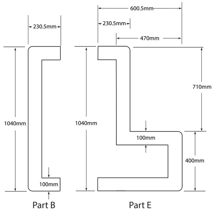
Backing board made up of 2 x sections (Part B) 230.5 x 1040mm and (Part E) 600.5 x 140mm and 4mm thick
