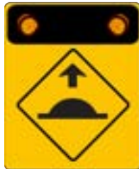
ROAD HUMPS AHEAD W3-4 A/B/C
