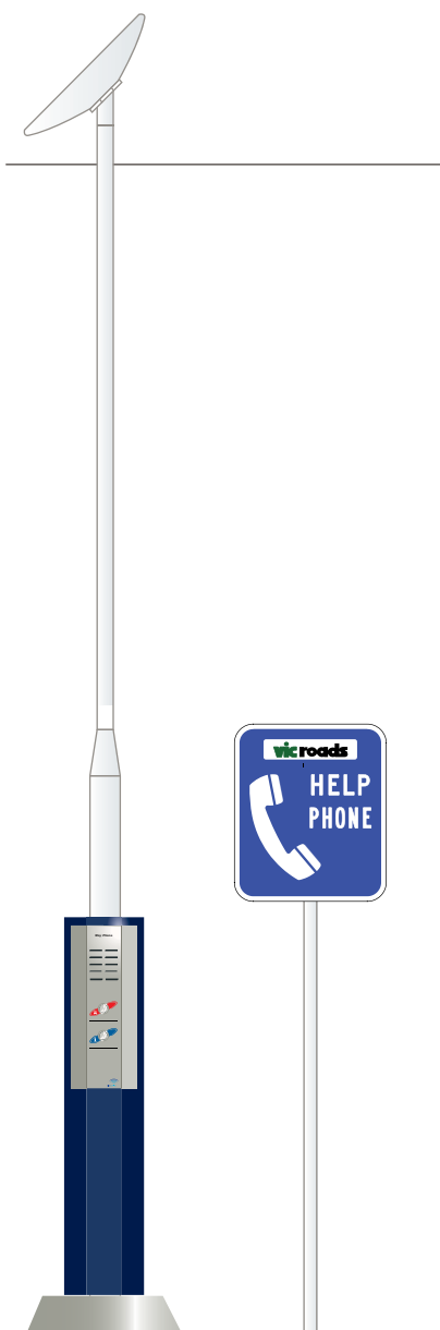
1375mm pedestal with 4m external solar pole
