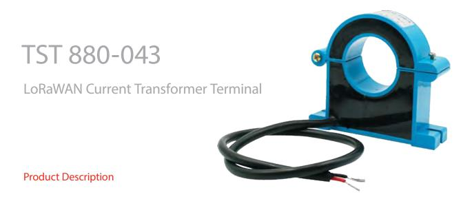
The current transformer is an instrument that converts the primary side large current into the secondary side small current according to the principle of electromagnetic induction. The current transformer consists of a closed core and a winding.
