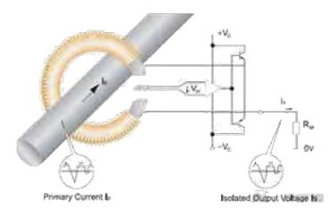
The magnetic flux generated by the current is concentrated in the magnetic circuit by the high quality magnetic core. The Hall element is fixed in a small air gap for linear detection of the magnetic flux. The Hall voltage output from the Hall device accurately reflects the change in current.
