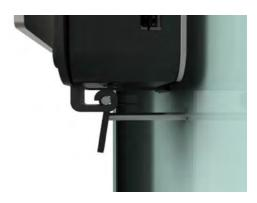
**3** Using the tool push the lever - this movement will override the lock disruptor
