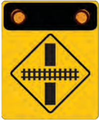
TRAIN CROSSING RIGHT ANGLE W7-8 A/B/C
