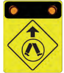
PEDESTRIAN CROSSING AHEAD W6-2 A/B/C
