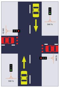
Mirrored lights on each side ensures visibility of eSTOP™ in multi-lane / highway situations or to prevent visibility being blocked by large vehicles.
