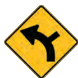
SIDE ROAD JUNCTION ON A CURVE
