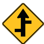
STAGGERED SIDE ROAD JUNCTION
